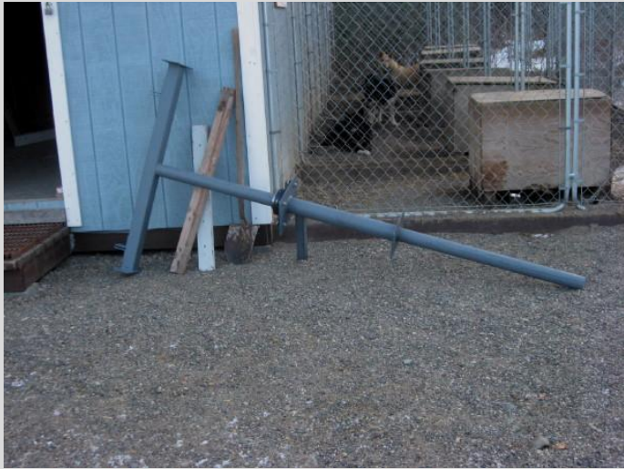
Azimuth A-Frame under construction. A-Frame revolves around Az-mast on eight dolly wheels
